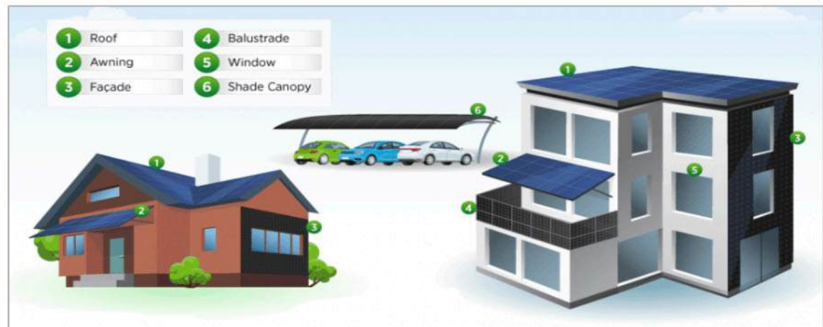
Figure 5.9 Examples of Building-Mounted Solar Systems Source: US Department of Energy
