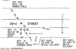
N1/4 CORNER SEC.25, T84N, R5E SET 1/2" REBAR w/ YELLOW CAP #14417
