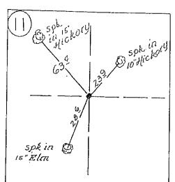
Set 1" Gas Pipe under 8"x6"×5' Limestone on line between '4 Sec Cors.
