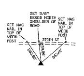
NE CUR, SE-SE, SEC. 8, T.87M, R.4E, OF THE 5TH P.M. PLACED 5/8"-STEEL-REROD-W/DRANGE-PLASTIC CAP MARKED "WEBER PLS 150841
