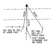
NW COR, SE-SE, SEC. 8, T.87N, R.4E.-DE-THE-5TH-R.M.-PLACED-5/8" STEEL REROD W/DRANGE PLASTIC CAP MARKED 'WEBER PLS 15084'.
