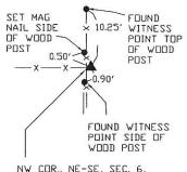
NW COR., NE-SE, SEC. 6, T.87N. R.4E. OF THE 5TH P.M. FOUND 1/2' DIA. REROD WYYELLOW CAP ND. 12642
