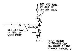
NV COR, NE-NE, SEC. 17, T.87N. R.4E. OF THE 5TH P.M. PLACED 5/8" REROD W/ORANGE PLASTIC CAP MARKED "WEBER PLS 15084"
