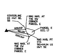
CENTER, SEC. 17, T.87N. R.4E. OF THE 5TH P.M. PLACED 5/8" REROD W/ORANGE PLASTIC CAP MARKED "WEBER PLS 15084"
