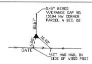
NW COR. SW-SW, SEC. 22, T.84N. R.2E. OF THE 5TH P.M. PLACED 5/8" REROD W/ORANGE CAP NO. 15084
