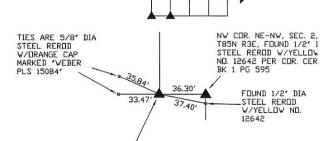
SE COR. OF THE SW-SW, SEC. 35, PLACED A 5/8" DIA STEEL REROD W/ORANGE CAP MARKED "WEBER PLS 15084"
