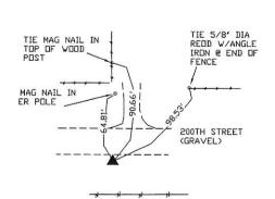
SW COR. SEC. 35, PLACED A 5/8" DIA STEEL REROD W/ORANGE CAP MARKED "WEBER PLS 15084"
