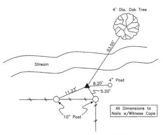
SE - SW 1/4 - NW 1/4 SET 1/2" REBAR W/ORANGE CAP #8419
