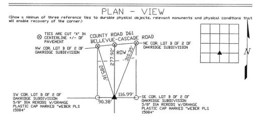
NE CORNER SE-SW SEC. 19 T.86N. R3E. OF THE 5TH P.M. PLACED 5/8' DIA. REROD W/ORANGE CAP MARKED 'WEBER PLS 15084'
