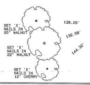
SW CORNER NE1/4, SE1/4, SEC.11, T86N, R3E SET 1/2" REBAR w/ YELLOW CAP #14417
