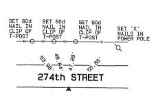
NW CORNER NE1/4, SE1/4 SEC. 11, T86N, R3E SET 1/2" REBAR w/ YELLOW CAP #14417
