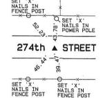
W1/4 CORNER SEC. 11, T86N, R3E SET 1/2" REBAR W. YELLOW CAP #14417
