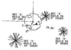
SE CORNER NW1/4, NW1/4 SEC. 23, T87N, R3E SET 1/2" REBAR W/YELLOW CAP #14417
