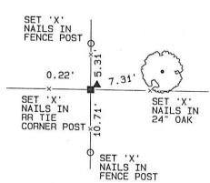
N1/4 CORNER SEC.18, T85N.R3E SET 1/2" REBAR W/ YELLOW CAP #14417
