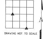
SE COR., SW-SE, SEC. 17, T.86N. R.2E. OF THE 5TH P.M. PLACED 5/8' DIA. REROD W/ORANGE PLASTIC CAP NO. 15084.
