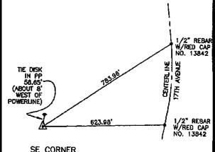
SE CORNER SECTION 31, T84N, R1E SET 1/2" REBAR W/RED CAP NO. 13842
