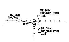
SW CORNER NE 1/4 SE 1/4 SECTION 31, T84N, R1E SET 1/2" REBAR W/RED CAP NO. 13842
