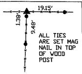
SW COR., NW-SE, SEC. 25, T84N RLE DF THE 5TH P.M. PLACED 5/8' DIA, REROD
