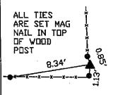
SE COR., NW-SE, SEC. 25, T84N RIE OF THE 5TH P.M. PLACED 5/8" DIA. REROD W/URANGE CAP NU. 15084.
