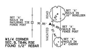
SE CORNER NW1/4, NW1/4 SEC.9, T84N, R3E FOUND 5/8" REBAR W/ CAP #14105
