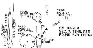
SET 60d SPIKE IN CLIP OF T-POST SET 'X' NAILS IN FENCE POST SET 'X' NAILS IN BRACE POST <sup>60</sup>.37.
