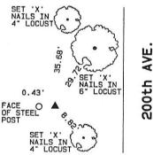
SW CORNER NW FRL 1/4, NW FRL 1/4 SEC. 7, TB4N, R3W FOUND 1/2" REB W/ CAP #10135 REBAR
