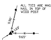
SW COR., NW-SW, SEC. 3, T.85N, R.4E, DF THE 5TH P.M. PLACED 5/8" DIA, REROD W/ORANGE PLASTIC CAP NO. 15084
