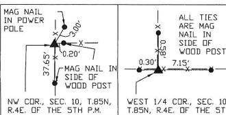
WEST 1/4 COR., SEC. 10, T.85N, R.4E. OF THE 5TH P.M. PLACED 5/8" DIA. REROD W/ORANGE PLASTIC CAP NO. 15084
