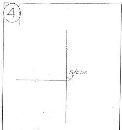
Set tron pin under 14" x 8" x 3" Limestone on NE side of Cor. Post
