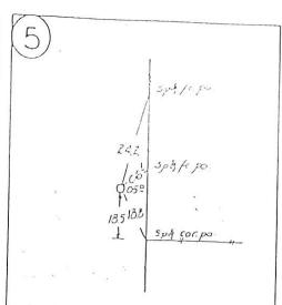
Set 17"x 10' x 6' Limestone on Line of 1/4 Cors. E & W and, No S. Cut "x' on Stone
