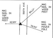
N 1/4, SEC. 18, T.84N. R.6.E DF THE STH P.M. PLACED A 5/8' DIA STEEL RERDD WJRRANGE CAP MARKED "WEBER PLS 15084" IN PAVEMENT
