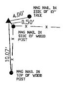
SE COR. SW-NV SEC. 28, T.85N. R.2.E OF THE 5TH P.M. PLACED A 5/8' DIA STEEL REROD W/ORANGE CAP MARKED "WEDER PLS 15084"
