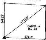
SV CUR., NV-NW, SEC. 22, T.85N. R.ZE. OF THE STH P.M. PLACED 5/8" DIA STEEL REROD W/ORANGE, PLASTIC CAP MARKED "WEBER PLS 15084"
