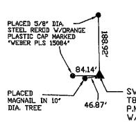
SW COR., SE-NW, SEC. 7, TB4N R4E OF THE 5TH P.M. PLACED 5/8" DIA. REROD W/ORANGE CAP NO. 15084
