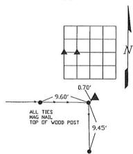
NE COR., NW-SW, SEC. 2, T.86N. R.1E. DF THE 5TH P.M. PLACED 5/8" DIA. REROD W/ORANGE MARKED " WEBER PLS 15084"
