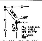
NV CDR., SV-NE, SEC. 12, TB6N R1E OF THE 5TH P.M., PLACED 5/8" DIA REBAR W/DRANGE PLASTIC CAP NO. 15084,
