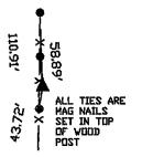
CENTER, SEC. 12, T86N R1E OF THE 5TH P.M., PLACED 5/8' DIA. REBAR W/DRANGE PLASTIC CAP NO. 15084.
