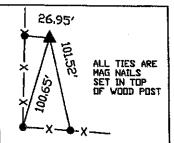
SE COR, SW-NE, SEC. 12, T86N RIE DF THE 5TH P.M., PLACED 5/8 DIA, REBAR W/DRANGE PLASTIC CAP NO. 15084.
