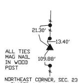
NORTHEAST CORNER, SEC. 23 - PLACED A 5/8' DIA STEEL REROD W/DRANGE CAP MARKED 'WEBER PLS 15084'
