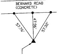
NW COR., SE-NW, SEC. 13, T.85N. R.1E. OF THE 5TH P.M. PLACED 5/8" DIA RERUD W/ORANGE CAP NO. 15084.
